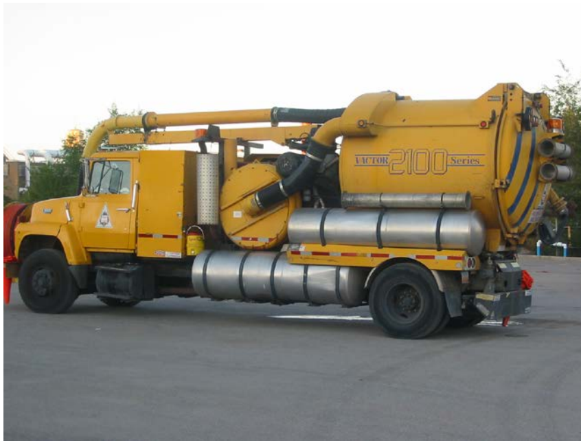
Combination Jet Cleaner and Vacuum Truck
