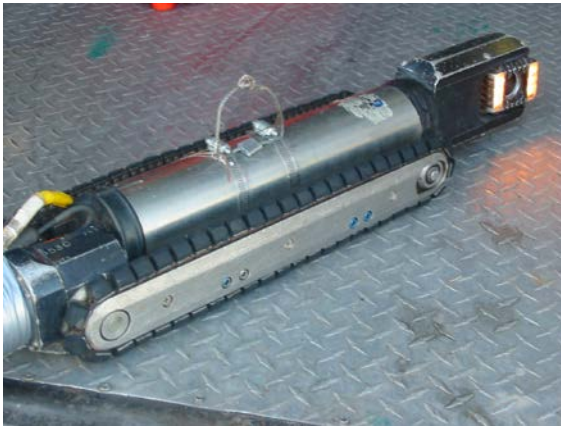
Tracked and 4-Wheel Drive Camera Systems with Rotating Camera Heads
