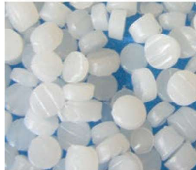
Adsorption Clarifiers use buoyant media in an upflow system design.
