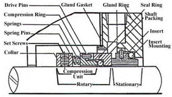
Figure 9.13 - Mechanical Seal Components
