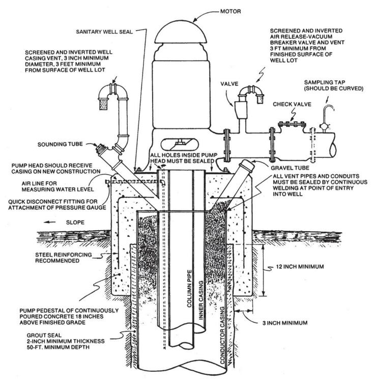
Figure 11.4 - Gravel Pack Well Construction
