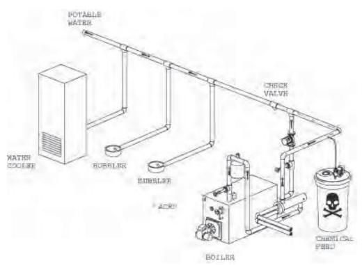
Figure 7.24 - Backpressure with boilers
