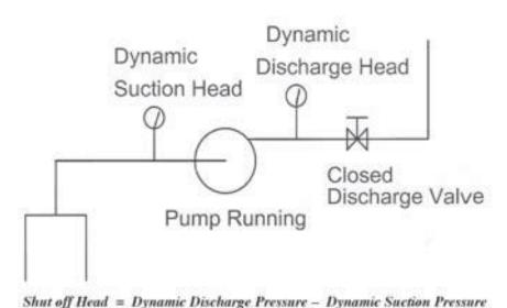
Figure 9.16 - How to Determine Shut-Off Head
