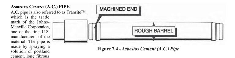
asbestos, silica sand and water onto a spinning anvil. The pipe is then shaped and placed in an autoclave to dry.
