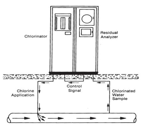
Figure 10.5 - Feedback Control Loop
