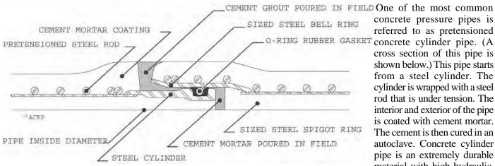
Figure 7.10 - Cross-section of Pretensioned Concrete Cylinder Pipe Joint
