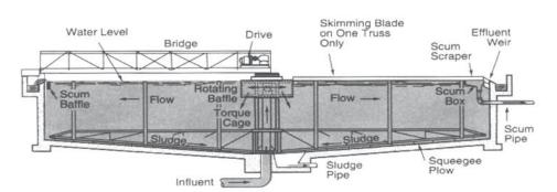
Figure 12.14 - Circular Sedimentation Basin
