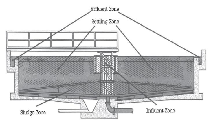
Figure 12.12 - Four Zones of a Sedimentation Basin
