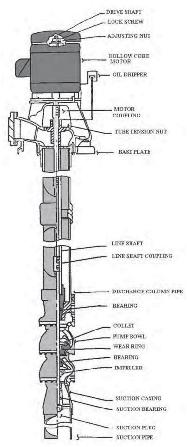
Figure 11.6 - Vertical Turbine Centrifugal Pump
