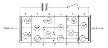
Figure 15.20 - ED Stack Demineralization Compartments (courtesy Ionics)
