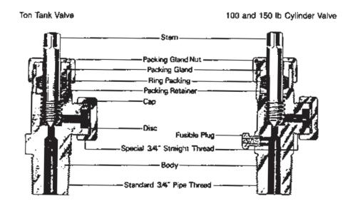
Figure 5.2 - Chlorine Cylinder Valve
