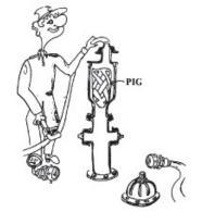
Figure 7.14 - Launching a Pig
