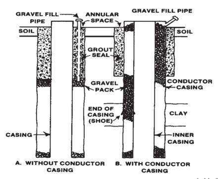
Figure 11.5 - Gravel Packed Well Types
