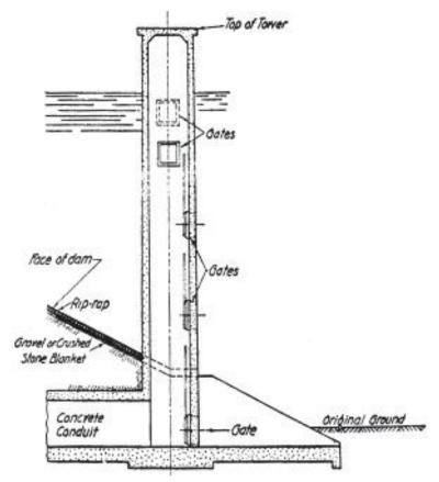
Figure 12.1 - Lake Intake Stucture
