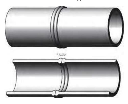
Figure 7.11 - HDPE Heat Fused Welded Joint
