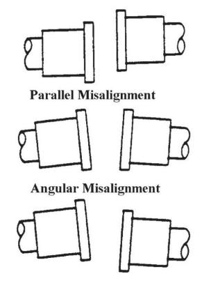
Usually a Combination of Both Figure 10.4 - Types of Misalignment
