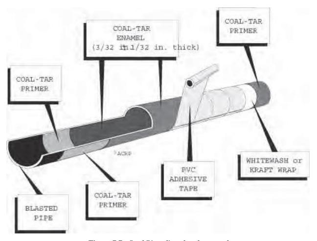
Figure 7.7 - Steel Pipe, dipped and wrapped
