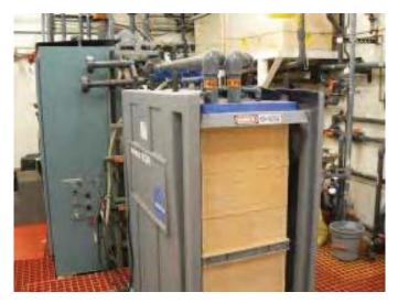
Figure 15.19 - Ionics Electrodialysis Reversal (EDR) Unit
