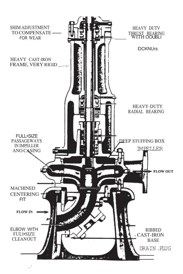
Figure 93-End-Suction Centrifugal Pump
