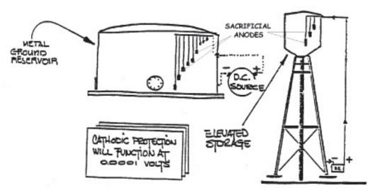
Figure 8.1 - Sacrificial Anodes Used for Cathodic Protection
