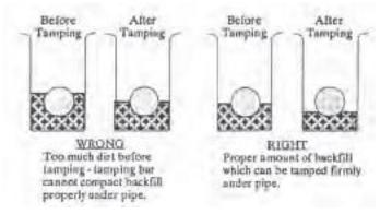
Figure 7.13 - Backfilling the Pipe
