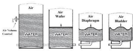
Figure 8.2 - Types of Pneumatic Tanks
