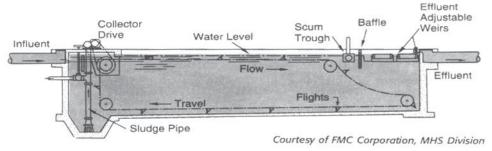
Figure 12.13 - Rectangular Sedimentation Basin
