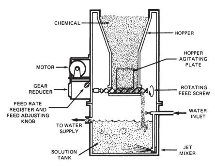
Figure 10.7 - Volumetric Chemical Feeder
