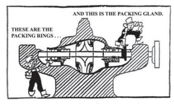
Figure 9.10 - Stuffing Material
