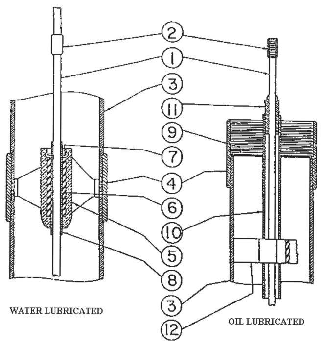
1 - Line Shaft 7 - Snap Ring 2 - Shaft Coupling 8 - Shaft Sleeve
