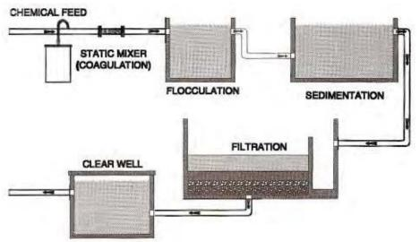
Figure 12.3 - Conventional Water Treatment Plant Diagram
