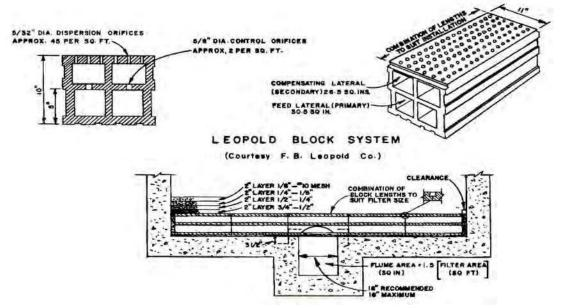
Figure 12.18 - Filter Underdrain System
