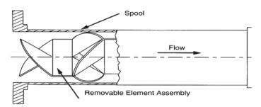
Figure 12.9 - Static In-Line Mixer
