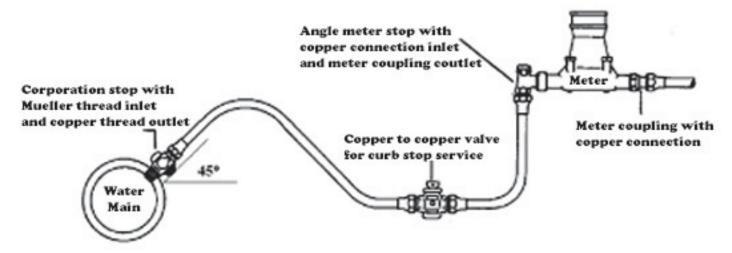
Figure 7.19 - Service Line Installation
