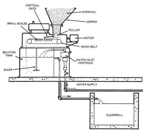
Figure 10.6 - Gravimetric Chemical Feeder
