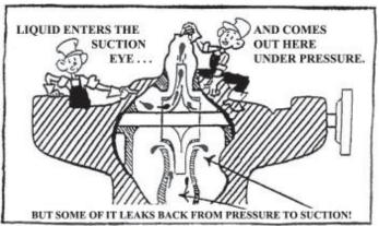
Figure 9.9 - Leak Back
