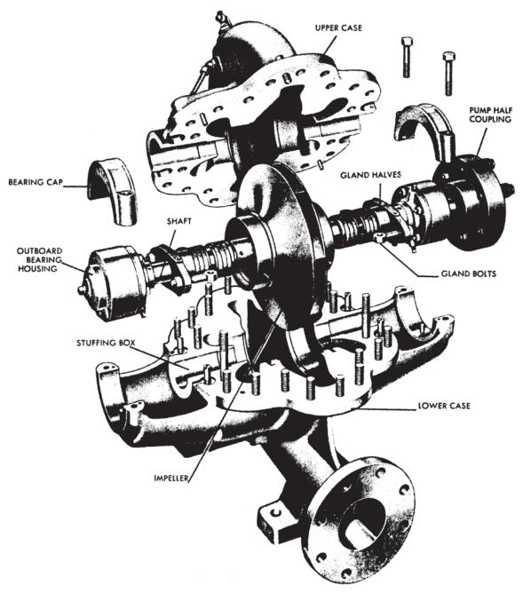
Figure 9.2 - Horizontal Split Case Centrifugal Pump
