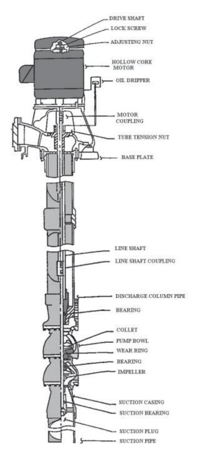
Figure 9.4 - Vertical Turbine Centrifugal Pump
