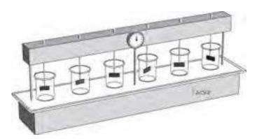
Figure 12.8 - Jar Test Apparatus
