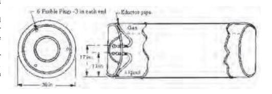
Figure 5.4 - Cross Section of a 1-ton Cylinder
