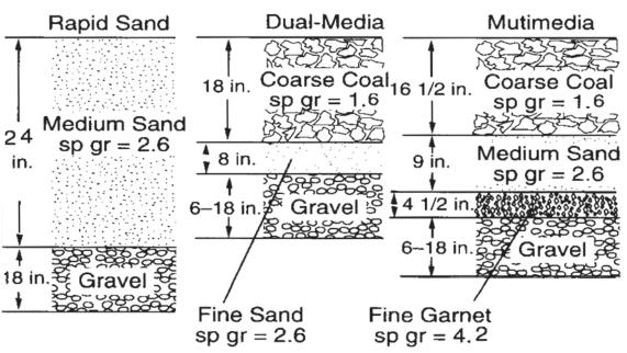
Figure 12.23 - Filter Media Configurations
