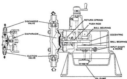
Figure 10.9 - Diaphragm Pump
