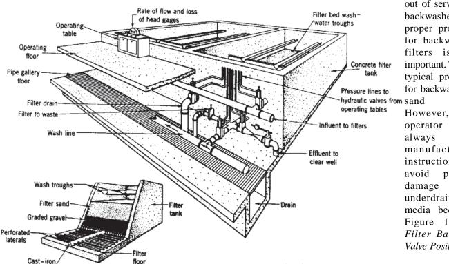
out of service and backwashed. The proper procedure for backwashing filters is very important. This is a typical procedure for backwashing a filter. However, the operator should follow manufacturer's instructions possible damage to the underdrain media bed. (See Figure 12.22 -Filter Backwash Valve Positions.)
