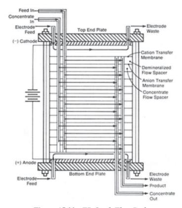
Figure 15.22 - ED Stack Flow Path (courtesy Ionics)
