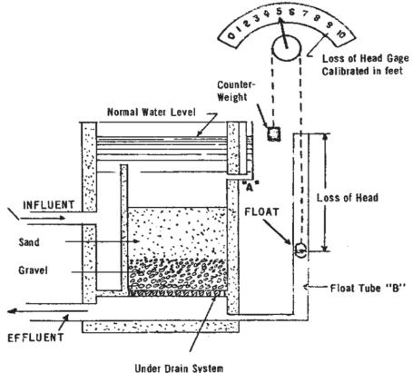
Figure 12.20 - Loss of Head Gauge
