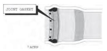
Figure 7.9 - PVC Integral Bell Cross-section
