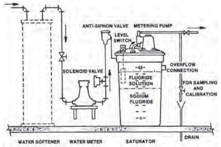
Figure 6.2 - Sodium Fluoride Saturator
