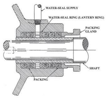
Figure 9.12 - Stuffing Box Cross-Section
