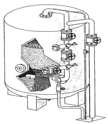
Figure 12.16 - Pressure Filter
