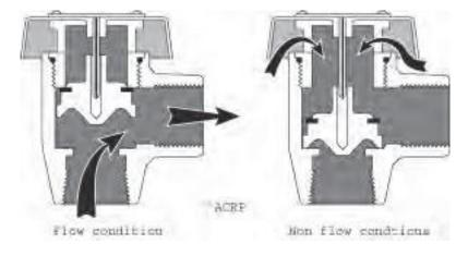
Figure 7.26 - Atmospheric vacuum breaker
