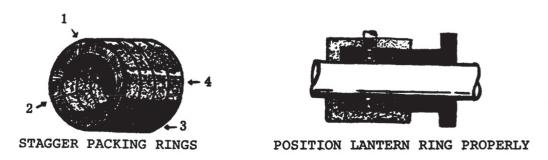
Figure 10.1 - Repacking A Pump
