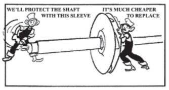
Figure 9.5 - Shaft Sleeve
