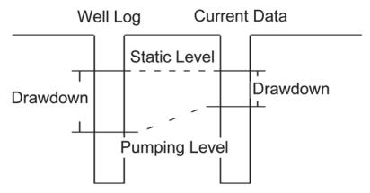
Figure 11.13 - Well Problem - Mechanical Pump
