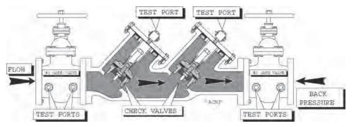
Figure 7.27 - Double Check Valve
