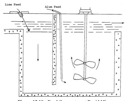
Figure 12.10 - Dual Compartment Rapid Mix
