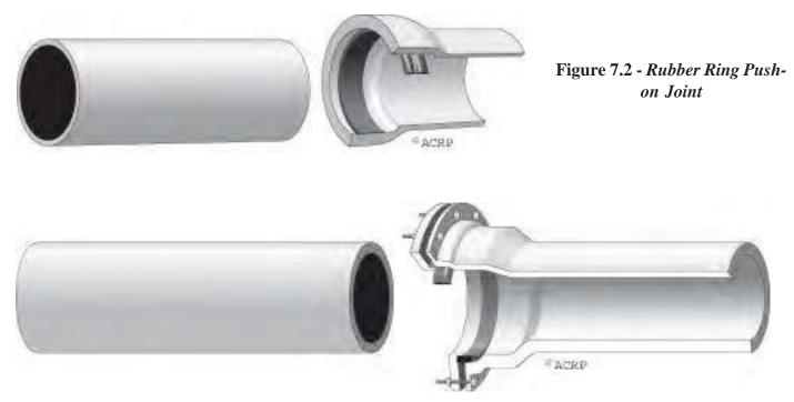
Figure 7.3 - Mechanical Joint
