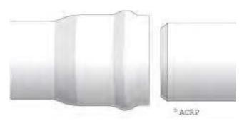
Figure 7.8 - PVC - Integral Bell & Spigot Joint
